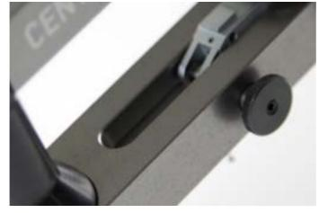
**Clamping:** With the two knurled screws, you can clamp the dial gauge quickly and precisely.
